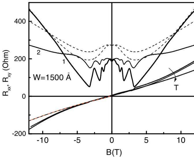
**Fig. 4** The longitudinal and Hall resistance as a function of magnetic field at  $\Theta = 89.6^\circ$  for different temperatures ( $T$ : 1.5 K, 4.2 K, 20 K, 30 K). Curve 1 shows magnetoresistance, when magnetic field is directed perpendicular to the current flow. Curve 2 shows magnetoresistance, when magnetic field is directed parallel to the current flow. Dashes –magnetoresistance at  $T = 20$  K and 30 K.
