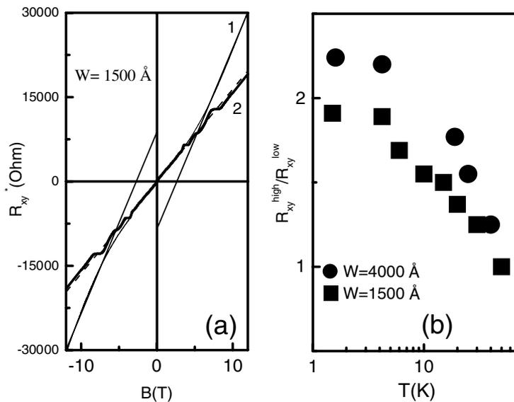
**Fig. 5** (a) Normalized Hall resistance at  $\Theta = 89.6^\circ$  (1) and at  $\Theta = 0^\circ$  (2) as a function of magnetic field,  $T = 1.5$  K. Dashes are the normalized Hall resistance at  $\Theta = 89.6^\circ$  as a function of magnetic field at  $T = 50$  K. The high field part of the curve 1 is prolonged until it cross the y axis. (b) The ratio between the slope of the Hall resistance at low and high magnetic field as a function of temperature for two samples.
