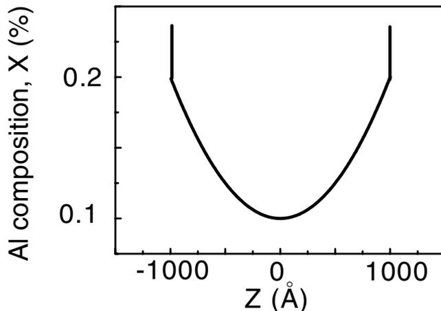
**Fig. 1** The variation of the Al composition in 2000 Å parabolic well along Z axis.
